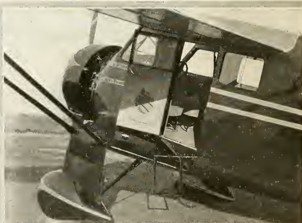
Cabin arrangement and new type landing gear of the new Stinson cabin monoplane shown on this month's cover of Aero Digest
